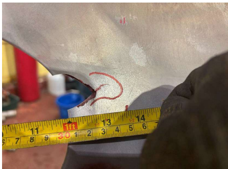
Indication #1 crack 1.25"x1"
